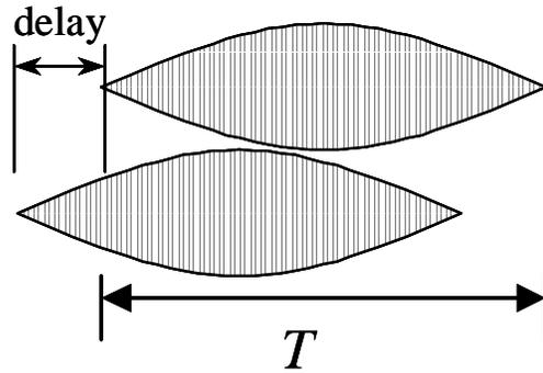
Fig. 3. PCC-OFDM symbol in a two-path channel
