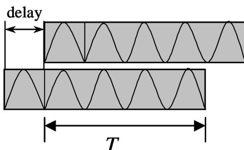
Fig. 2. OFDM symbol in a two-path channel
