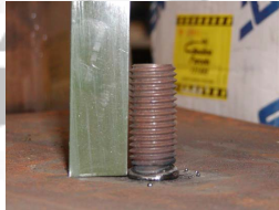
Nelson Stud after welding
