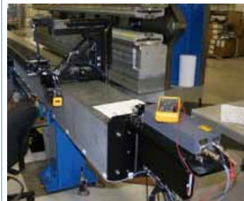
PAL Magnetic Field Measurement System
