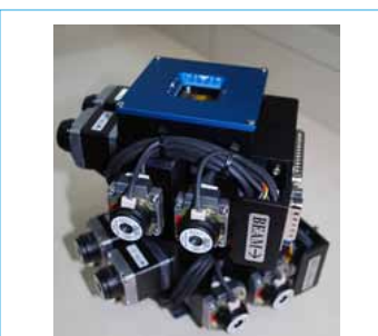
APS Two Slanted 30 Degree Slits
