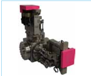
SwissFEL High Precision Slits (Curtain Design)
