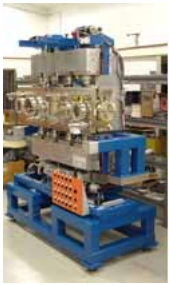
BNL Cryo In-Vacuum Undulator
