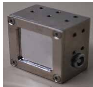
X-Ray Beam Monitor (XBM)
