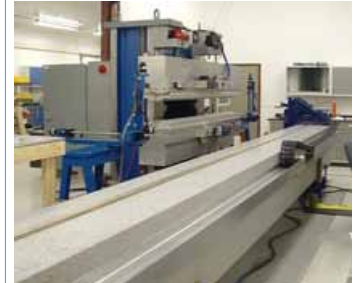
ADC OLD In-House Undulator Magnetic Measurement System
