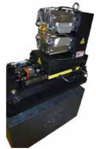
NSLS II Three-Pole Wiggler - TPW
