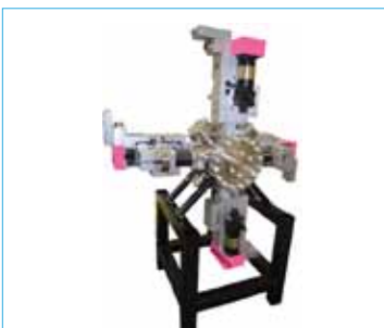
UHV Slit System for ESRF
