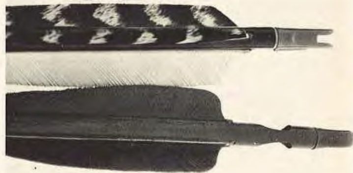
Above: Shaft at top is standard arrow and may be used with longbow or Fist-Flite , while shaft at bottom has been modified to shoot in the Wrist Rocket . (Left) Nicolasi checks nock before trying shot with a Fist-Flite .
