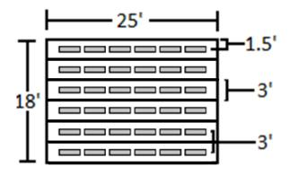
If designed as a conventional trench formation, the resulting footprint would be approximately 1,500 ft<sup>2</sup>. The above PPBPS bed formation offers a 70% reduction in area needed on the lot.
