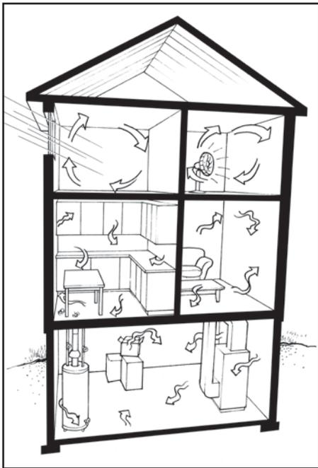
**Figure 3** Circulation of air in a house
