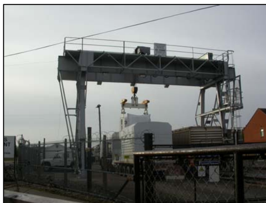
TRANSFER OF AGR FLASK FROM ROAD VEHICLE TO TRAIN FLATROL SLIDE BACK COVERS ON BOTH TRUCK AND FLATROL
