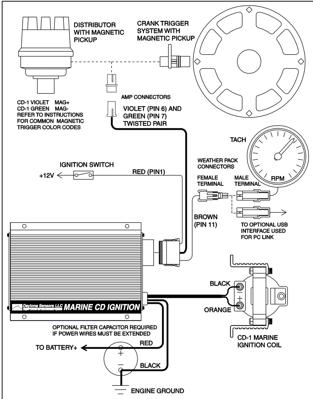
Figure 3 – Basic Mercury Marine Hall Effect Distributor Hookup
