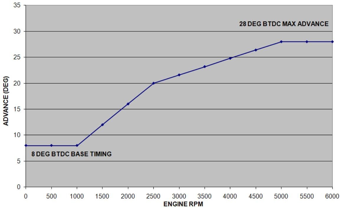
**NORMALLY ASPIRATED ENGINE TIMING CURVE**
