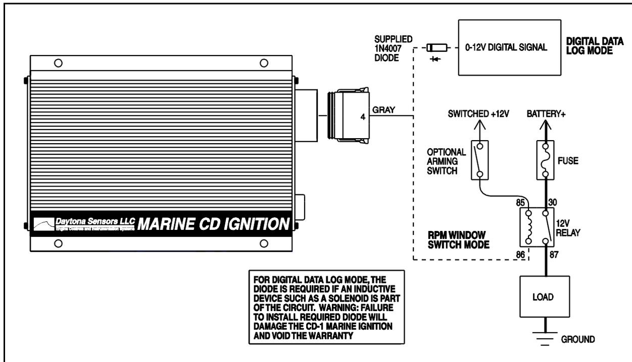
Figure 9 – GPIO3 Data Logging Hookup Options
