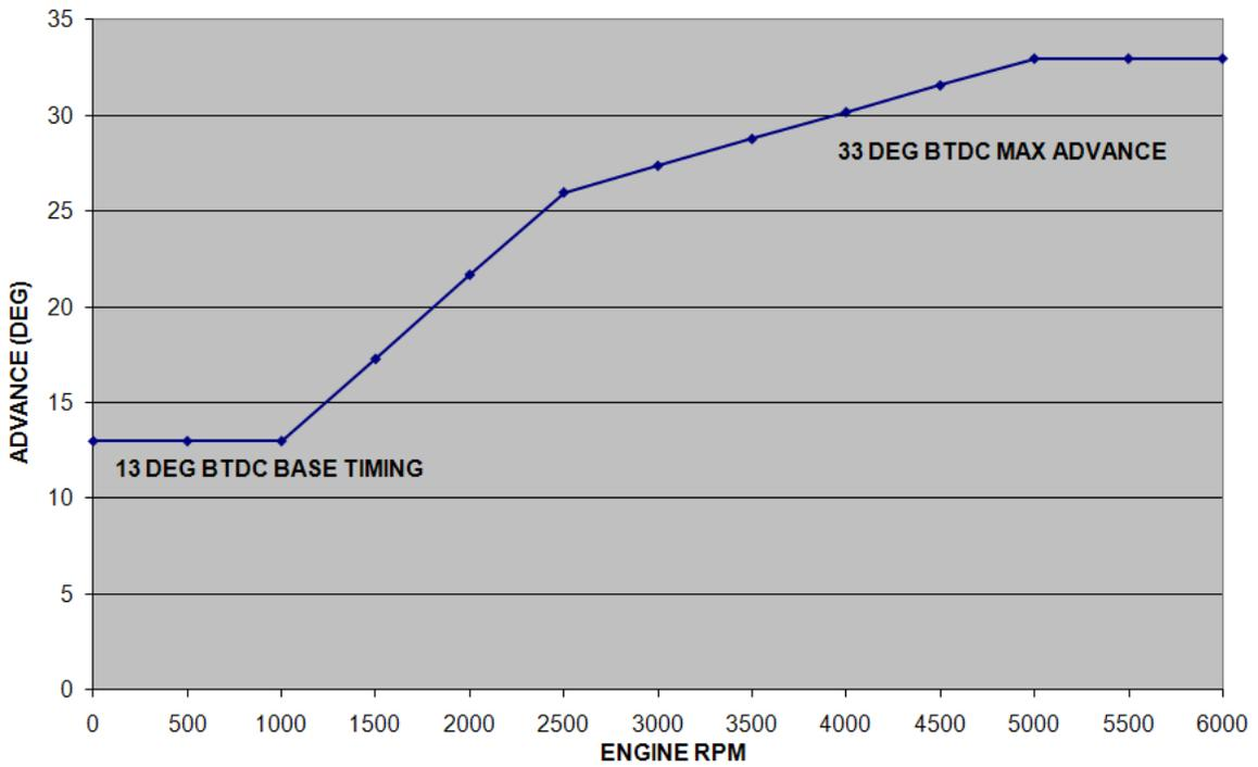
**MERCURY HP600SC FIREPOWER TIMING CURVE**
