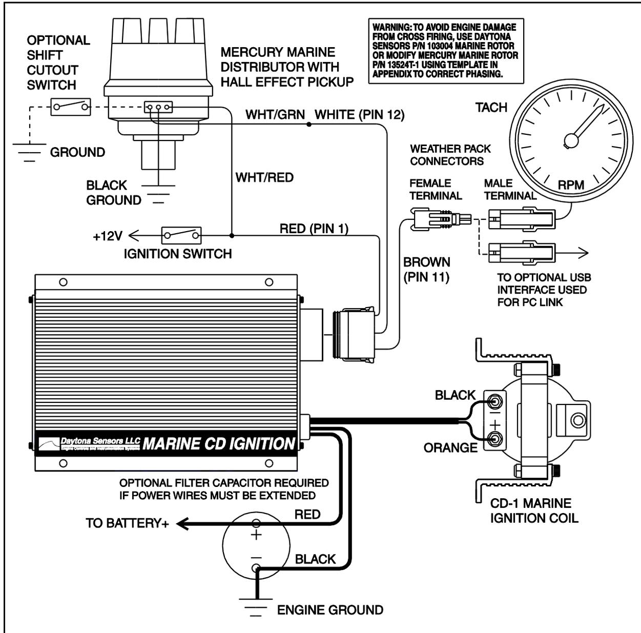
Figure 4 – Basic Module Trigger Hookup
