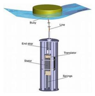
Fig: Schematic Diagram of Buoy.
