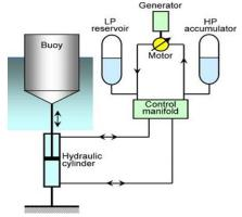
Fig: Block Diagram of the system.
