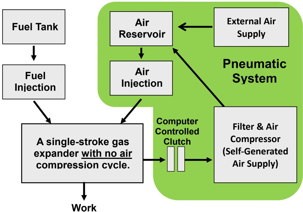
**Fig. 1: FAI is a combination of an engine and an air motor.**
