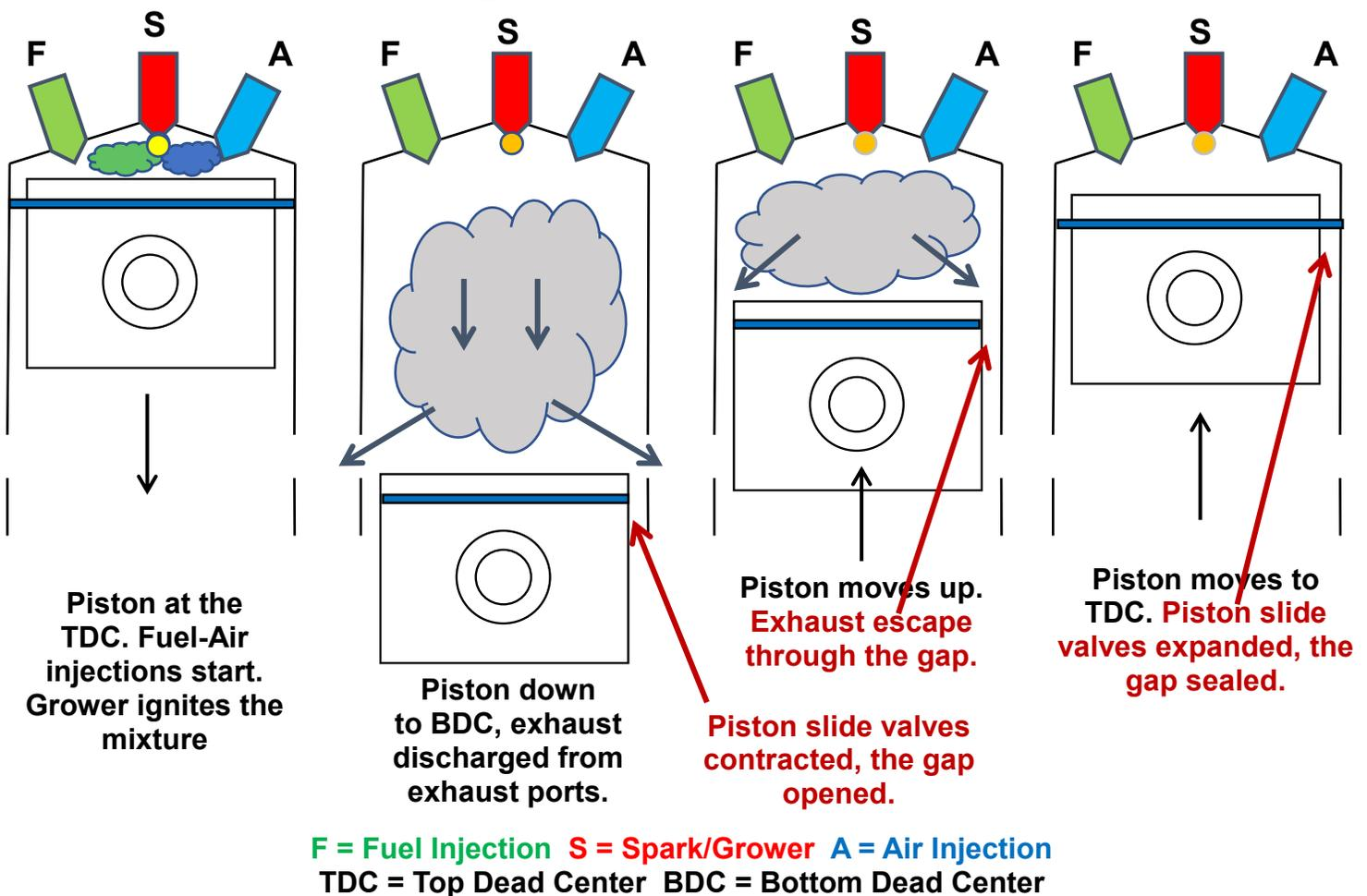
Fuel-air injection timing and amount are programmable; combustion completeness and stoichiometric ratio are defined by software look up table and executed by digitally controlled injectors (ref. US patent 9121337, 9677468). Fuel can be liquid or gas phase such as alcohol, gasoline, diesel, eFuel or methane, propane, butane, etc.
