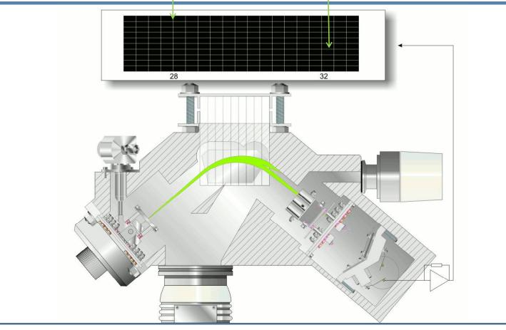
The abundance of selected ions is directly proportional to peak height. It is not necessary to measure the peak in the dead center (i.e. quadrupole MS). The entire peak top yields the same result.
