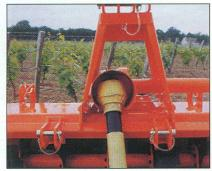
The Rotavator can be operated in line or offset on the right-hand side by simply repositioning the sliding clevis brackets.
