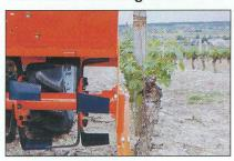
The blades on the rotor extremities face outwards (44"/56") to ensure the maximum working width in relation to the overall width of the Rotavator enabling close working to inrow plantations.
