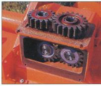
The HR 20 can be equipped with a single speed gearbox which gives a rotor speed of 200/min at 540/min PTO. The versions with Selectatilth gearbox can be set to rotor speeds of 165-190-215 or 235/min at 540/min PTO.
