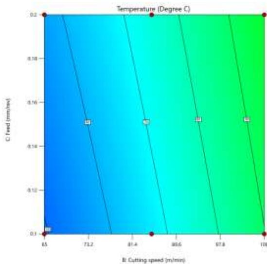
Figure 5: Interaction effects of temperature on cutting speed and feed
