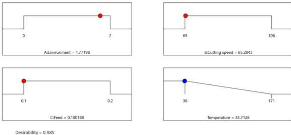
Figure 9. Optimum desirability ramp graph for all the input and response
