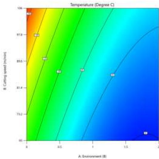
Figure 3: Interaction effects of temperature on environment and cutting speed
