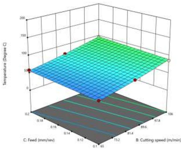
Figure 8. Variation of temperature against cutting speed and feed
