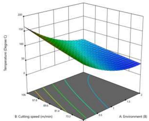
Figure 6: Variation of temperature against environment and cutting speed
