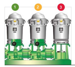
Example illustrates a three 100 hp high efficiency pumping system with EBV and VFD control configuration.
