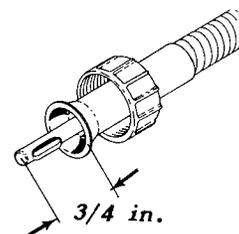
*Tip projection of completed core.*
