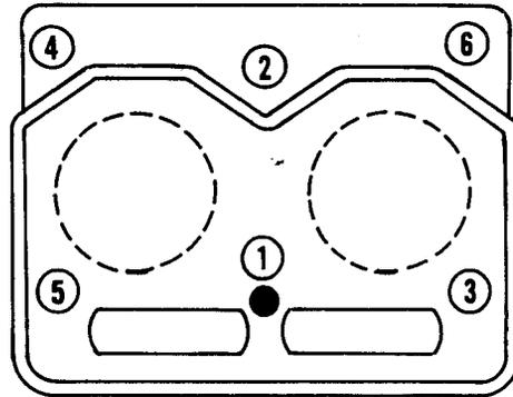
*Cylinder Head Tightening Sequence.*
