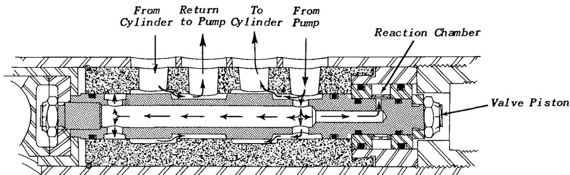
*Fluid Flow Pattern with Actuating Valve Piston in Turning Position*
