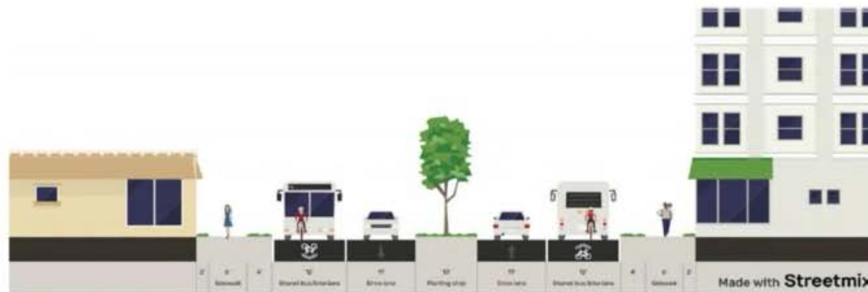
Figure 2- Proposed BAT Lane Cross Section at Douglas Street
