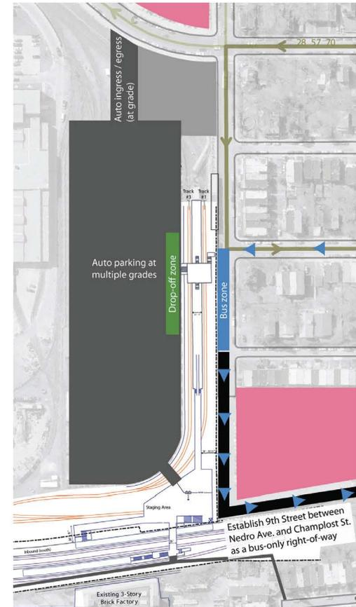
**Reconfiguration Option 3:** buses rerouted (**blue**) to 10<sup>th</sup> → Nedro → 9<sup>th</sup> (new bus-only ROW along 9<sup>th</sup> Street between Nedro and Champlost); auto access to garage is from 11<sup>th</sup> Street (both park-and-ride and **drop-off**)
