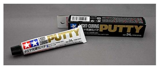
I just tried the new Light Curing Putty (No. 88888) from Tamiya. And this stuff is very cool! It's a translucent yellow-orange polymer that acts like regular contour putty. You trowel it over the area to be filled, smooth it out, and can work it for a while. Then the magic can begin. To harden it, you only need to expose it
