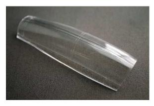
Remember these rules: start small and work in a circle (as you progress with finer grits, you'll need to increase the area you're sanding), always rinse off the residue between grits (you don't want any coarser residue when progressing), and work any liquid or paste polish until dry, then clean. If you're satisfied with the clarity of the piece, move on to the final stage: Back to the Future.
