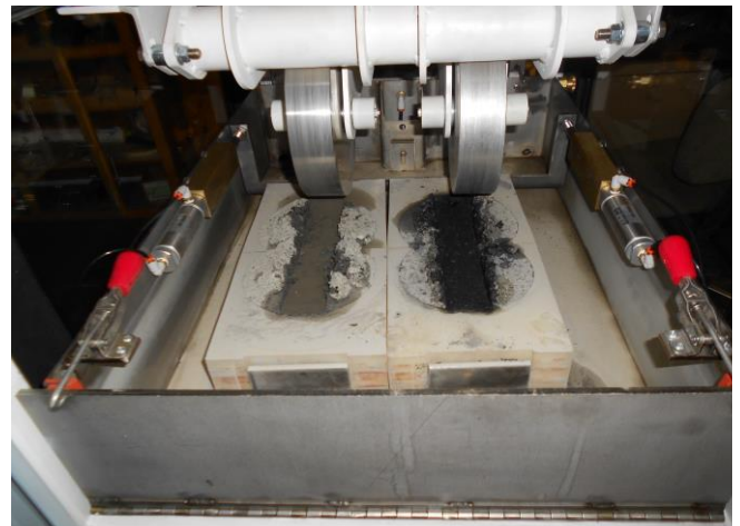
Completed Hamburg Test with Gyrotory Samples
