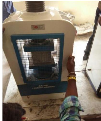
**Fig,2 Compressive testing set up**
