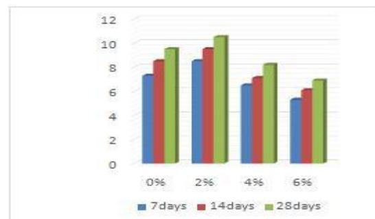
Chart 3: Flexural strength on various concrete ratio
