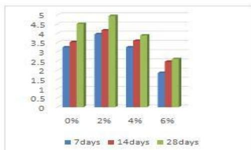
Chart 2: Split tensile strength on various concrete ratio
