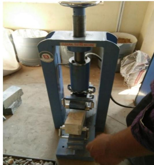
Fig No: 4 Flexural Test set up
