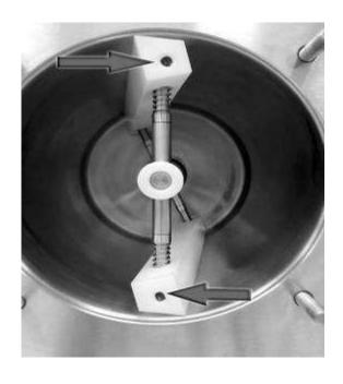
After the dasher is in place, you should be able to see the "dimple" on each of the two blades BEFORE you put the front door in place (see photo). If this is wrong the machine will not properly. You operate need to be aware of this Each and Every time you assemble the machine.
