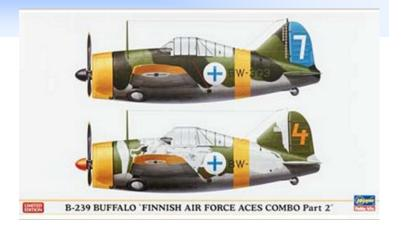
The B-239 Finnish Brewster Buffalo was an export version of the F2A-1 U.S. Navy Buffalo that was de-navalized by removing the tailhook, life-raft containers, cockpit armor and not having self sealing fuel tanks. They were then equipped with a lower horse power engine. All of these changes made for a lot lighter and maneuverable aircraft.
