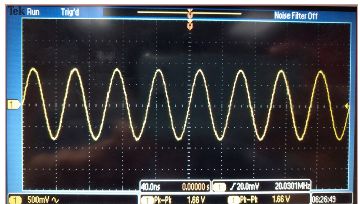
Figure 15. Impedance is mainly capacitive at 20 MHz
