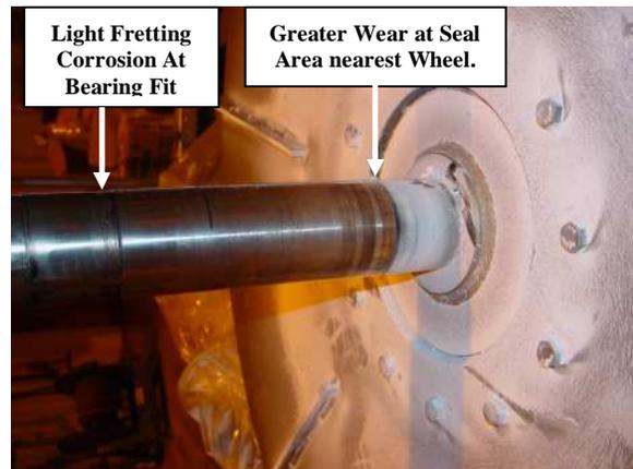
**Figure 11. Fan Rotor Removed From Service.**
