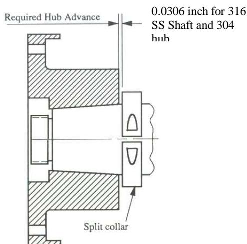
The specific fan hub advance required to provide adequate interference fit at operating speed and temperature calculated to 0.0306 inch, **Figure 29**.
