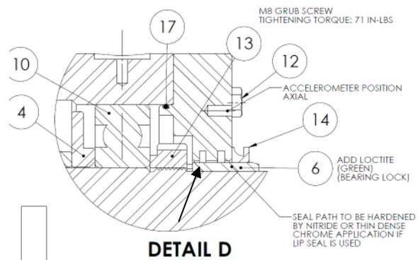
**Figure 22. Detail of Coupling End of Bearing Housing Showing Seal and Seal Path.**
