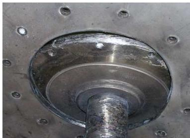
**Figure 6. Fan Shaft and Fan Hub. Shaft Heavy Rub Against Fan Wheel.**
