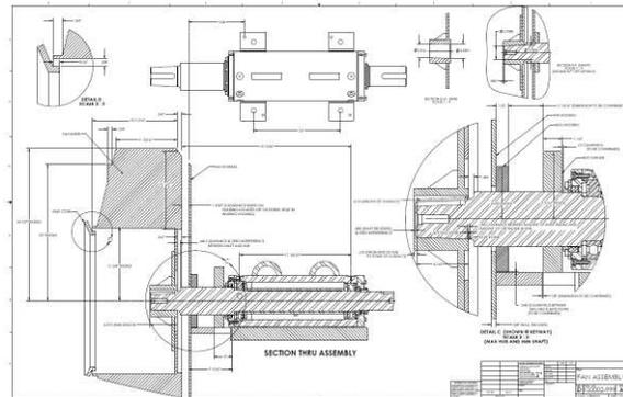
**Figure 27. Bearing Housing, Shaft, Fan and Bearing Support Plate Drawing.**
