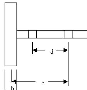
**Figure 33. Schematic of Fan Rotor For Balance Calculations.**
