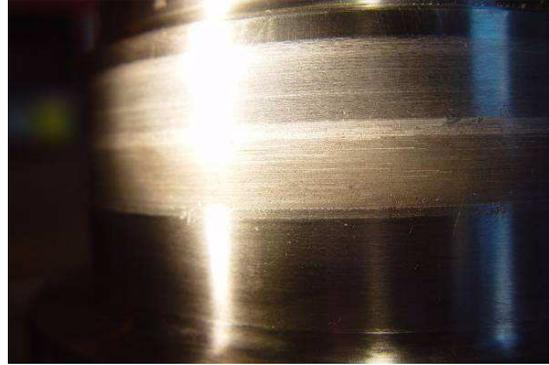
**Figure 32. Journal Showing Balance Machine Roller Damage to Bearing Fit, Wheel End. This Roller Track Appeared Wider or the Shaft Shifted Axially During Balancing Operation Generating Two Tracks.**
