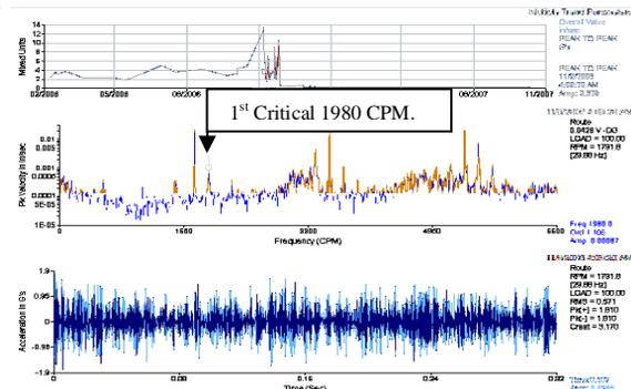
**Figure 13. Fan Inboard Bearing Horizontal, High Resolution Spectrum, Rotor & Bearings Changed After Nov 5, 2006 Outage. Rotor 1<sup>st</sup> Critical Shifted to 1980 CPM.**
