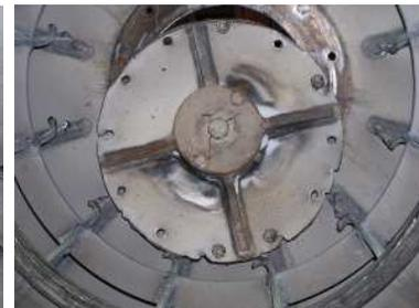
**Figure 7. All Fan Wheel Hubs Failed.**
