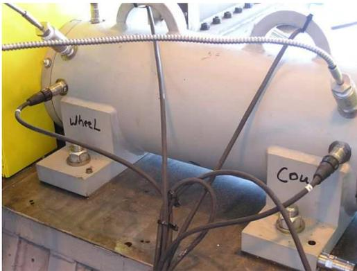
**Figure 36. Close Up Photo of Newly Installed One Piece Bearing Housing With Accelerometers and Temperature Sensors Installed.**
