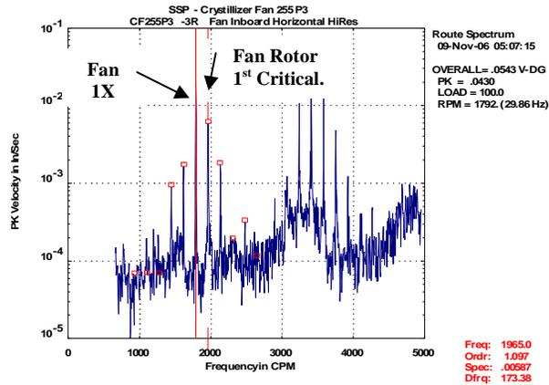
**Figure 2. Spectrum at Fan Inboard Brg Horizontal Shows Fan Rotor 1<sup>st</sup> Critical at 1965 CPM, 173 CPM Above Running Speed. Sidebands About 1X and 2X Run Speed are Modulated by the Fan Rotor 1<sup>st</sup> Critical Frequency.**
