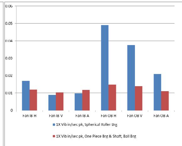
**Figure 40. Chart Fan 1X Vibration in/sec pk Modified Bearing Housings & Shaft.**
