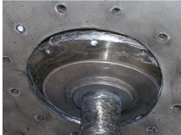
**Figure 30. Nov 6, 2006 Failure, All Fan Hub Bolts Failed.**
