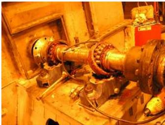
**Figure 3. Image Taken Shortly After Fan Failure.**
