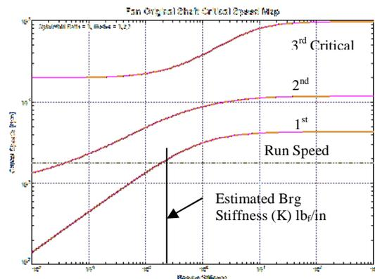
**Figure 14. Undamped Critical Speed Map for The Original 3-3/16" Fan Rotor.**
