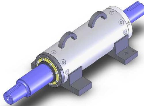
**Figure 20. 3D Model of Bearing Housing and Shaft.**
