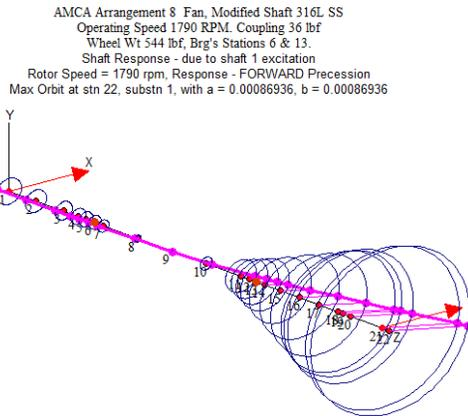
**Figure 17. Shaft Damped Unbalanced Response to G2.5 Balance Quality Grade at Run Speed.**
