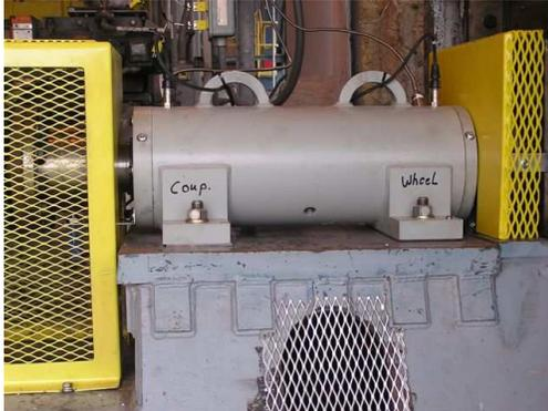
**Figure 34. Photos of Newly Installed One Piece Bearing Housing.**
