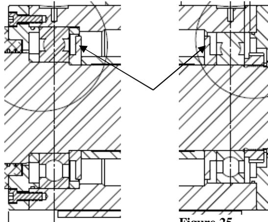
**Figure 24. Grease Dam at Fan end of Brg Housing.**
