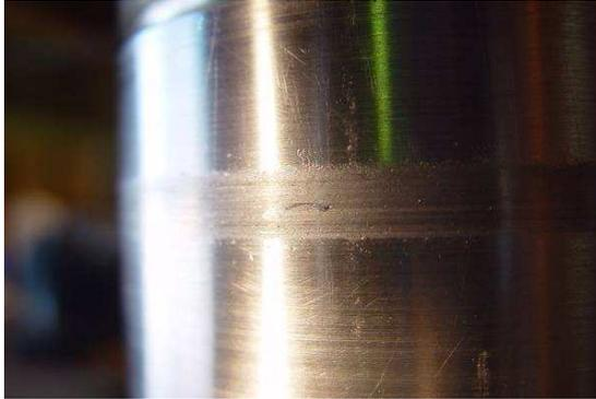
**Figure 31. Journal Showing Balance Machine Roller Damage to Bearing Fit (Coupling End). Metal Shaving Embedded in Journal.**
