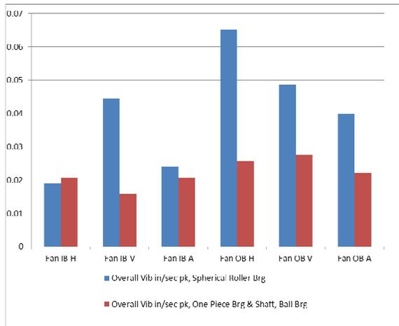
**Figure 39. Chart Fan Bearing Overall Vibration Original Design and Modified Design.**
