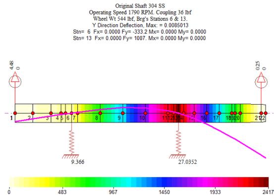
**Figure 18. Static Bending Stresses, OEM Shaft 304SS, Maximum 2417 psi at Wheel End Bearing.**
