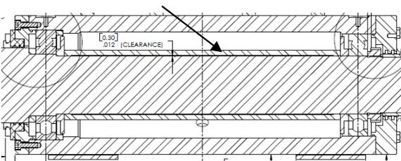
**Figure 26. Bearing Spacer Sleeve.**
