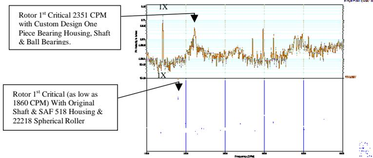
**Figure 38. Frequency Spectra at Fan OB Brg Housing, Hor, Original Shaft & Bearings Top Plot, New Design Brg Housing and Rotor Lower Plot.**
