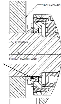
**Figure 21. Seal at Fan End of Brg Housing.**
