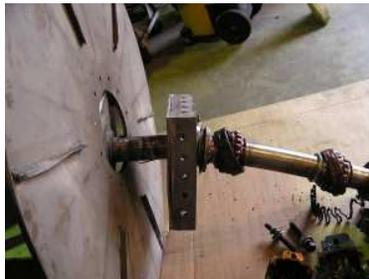
**Figure 4. Fan Shaft and Wheel in Shop After Failure.**
