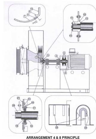
**Figure 1. AMCA Arrangement 8 Fan Drawings.**
