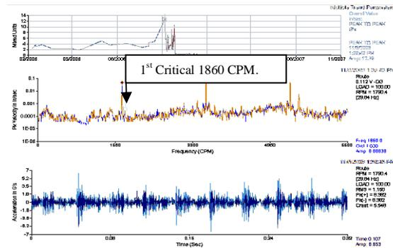
**Figure 12. Fan Inboard Bearing Horizontal, High Resolution Spectrum, Just Before Shutdown November 5, 2006.**
