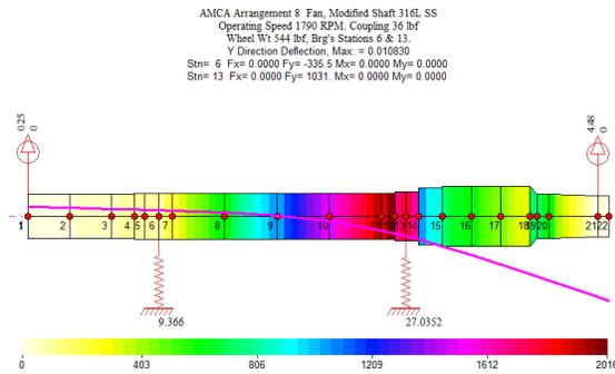
**Figure 19. Static Bending Stresses, New Shaft Design, 316L SS, Maximum 2016 psi Inboard Wheel End Brg.**
