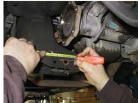
12. Now, you will need to grind 1/4" off of the lower a-arm pockets in each corner. If our piece doesn't fit exactly then you may need to grind a little more off (each frame varies slightly)
