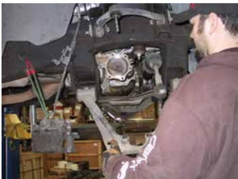
8. Take off the front skid plate w/ shield. Uninstall the driveshaft from the differential. Unbolt the rear crossmember (this is the crossmember that the a-arms hook to).
