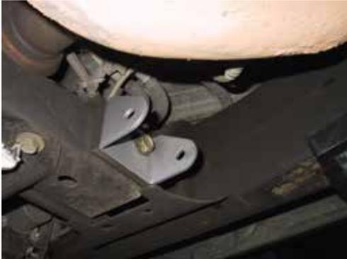
31. On the backside of the rear crossmememmer, there is one hole to bolt the new U bracket for the compression strut. Using the new **compression struts** and the provided 1/2" x 4 1/2" bolts and hardware, bolt to the tabs. Depending on the exhaust your vehicle has and how it is ran, you may need to modify the exhaust for clearance.
