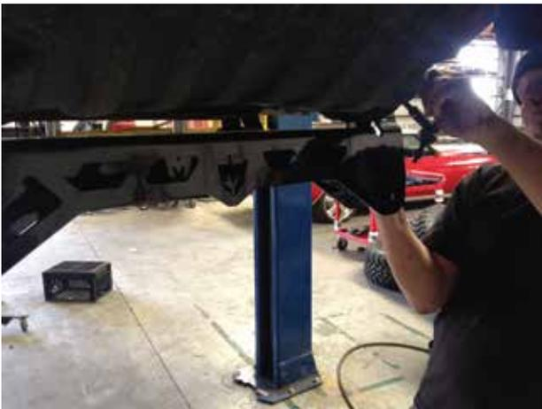
18. Install the lower a-arms into the new McGaughy's crossmembers with the supplied 5/8" x 5" for the front pocket.
