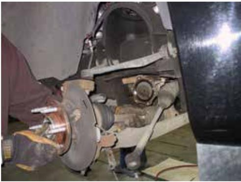
5. Unscrew the factory ball joint nuts from the ball joints and then use a rubber mallet to hit the spindle so that the ball joints can be removed. Be very careful to only hit the spindles and not the ball joints.
