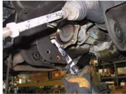
11. On the PASSENGER side lower a-arm frame mount you will need to cut off 3 1/2". Using a marker and a straight edge, measure and mark 3 1/2" from the edge of the frame mount inward and then cut with a sawzall.
