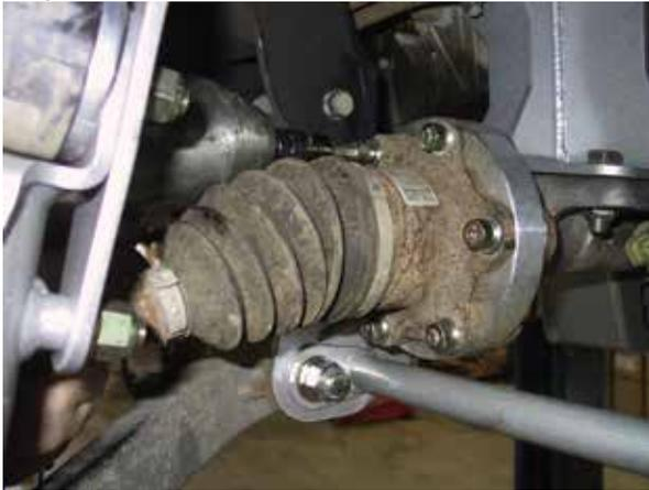
24. Using the factory hardware, install the factory hubs/bearing assembly (torque to 125 ft. lbs.). Install the factory rotors and then the calipers and torque to 30 ft. lbs.
