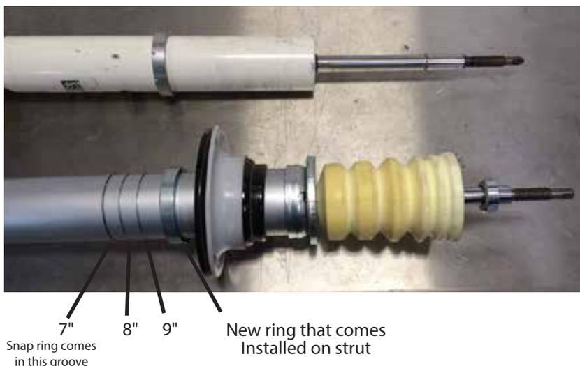
Installing the factory spring & Inner bump stop cup to the new McGaughy's strut.
