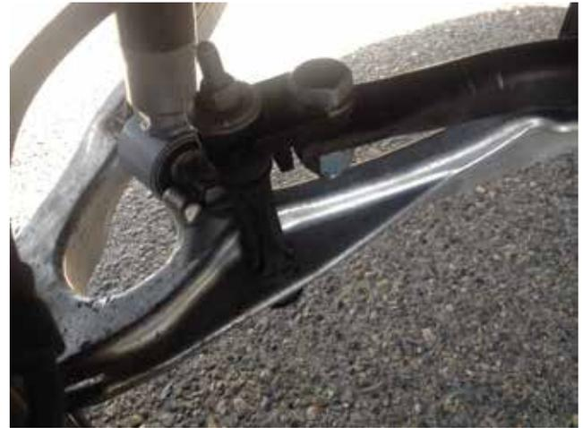
27. Bolt the McGaughy's **front brake line bracket extender** to the factory mount using the original hardware and then bolt the original bracket to the new extension bracket using the provided 1/4" hardware.
