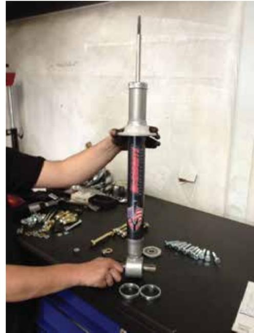
21. Install entire strut assembly onto the vehicle.
