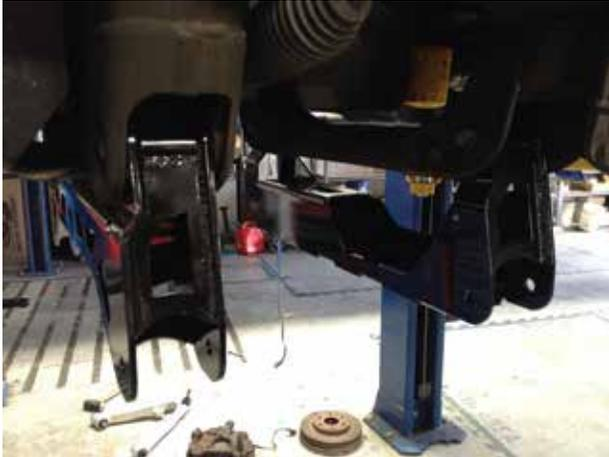
17. Install the McGaughy's front crossmember drop using the factory hardware into the lower a-arm pockets. (don't tighten yet)
