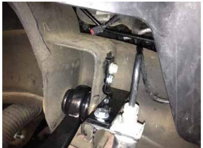
28. Use the provided 1/4" x 3/4" bolt and hardware to bolt the factory brake hose and the ABS line to the new lift spindle. Connect the ABS line back together and use wire ties to secure the ABS line out of the way of anything including the tire/wheel. Check for clearance and be sure there is enough slack for when the suspension travels.
