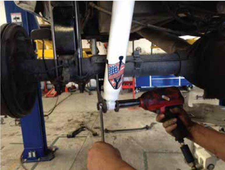
38. Make sure the factory ABS line has enough slack so that when the rear-end is at its fullest downward travel, the line isn't stretched. Wire tie the ABS line to the U-bolt and anywhere else needed to keep it out of the way for clearance, again making sure there is enough slack.
