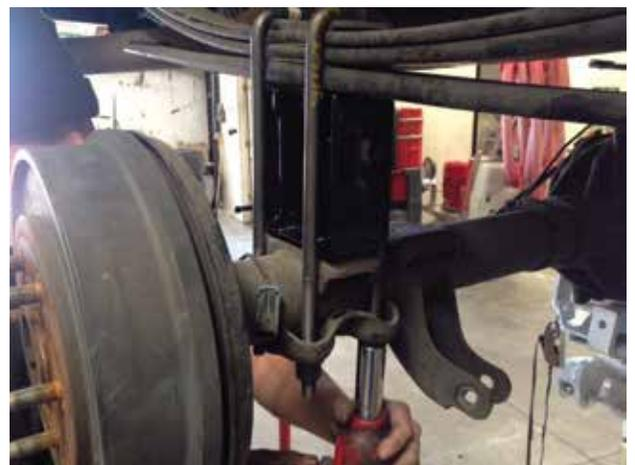
36. Using the provided self drilling hex head screws, re-route the factory brake line bracket from the top of the frame to the underside of the frame. Check for clearance.
