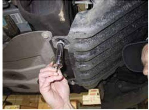
9. Uninstall the two clamps, vacuum line, and electrical plug from the differential housing and then remove.
