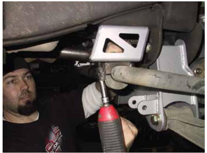
26. Install the new **sway bar extenders** to the bottom of the sway bar with the short side of the extender on the stop plate end using the provided 18mm hardware (torque to 110 ft. lbs.) Install the factory sway bar end links to the sway bar extenders and to the lower a-arms.
