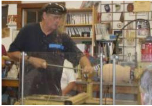
Nigel makes a center cut in the hollowform in preparation to hollowing around it. He goes in just an inch or two at a time.
