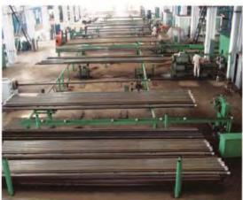
Four production lines for pre-stressed insulated tubing/casing will provide specialized production with high efficiency.
