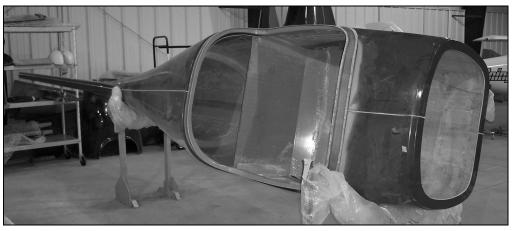
Figure3 fuselage shell
