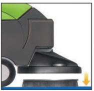
Spin-on/Spin-off Brush Pad Automatic brush attachment and release system (without hands or tools).
