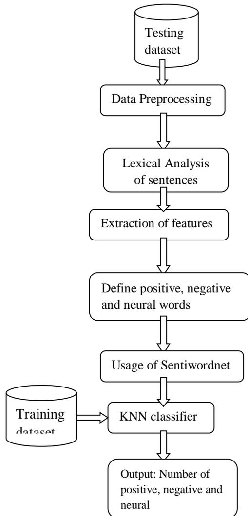
Fig.1:Proposed System Architecture
