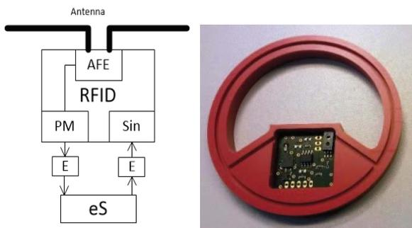
Figure (b) RFID sensor system scheme (left) and system design with circular HF antenna (right)
