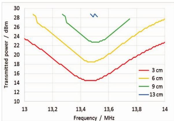
Figure (e) Exemplary results of HF measurements for RFID systems at different installation depth
