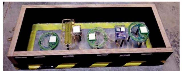
Figure (c) Test specimen with RFID systems before filling with concrete.
