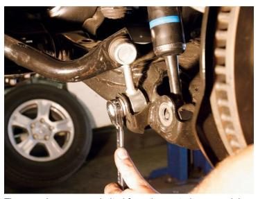
The sway bars were unbolted from the control arms and then the coilovers were removed.
