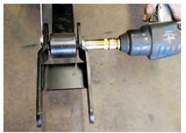
The shackles that attach the leafs to the frame were removed, as well. Notice the OE and longer aftermarket shackles compared to each other. The new shackles were bolted onto the ends of the leaf springs. There were two sets of bolts on the parts of the shackles that attach to the frame, which give the option to go low or lower. We chose lower.
