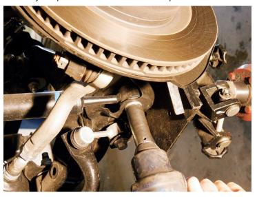
Starting with the front suspension, the coilover assembly was unbolted.
