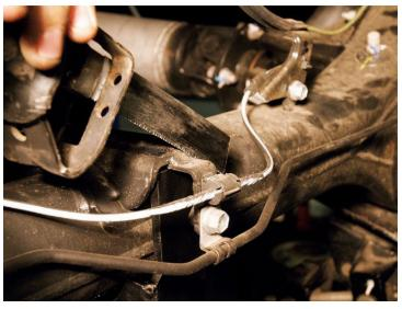
The mounting points for the brake lines and sensor wires interfered with the fitment of the aftermarket bump stops, so they were sawed off and the brake line and sensor wire were later attached to the new bump-stop assemblies that were secured to the top of the axle with the aftermarket U-bolts.
