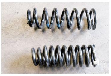
Here, the factory coil is lying next to the McGaughys shorter aftermarket coil. The new spring was installed into the coilover assembly, then the front suspension was put back together.
