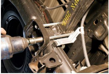
Moving on to the rear suspension, what we had was a flip kit where the axle was moved from below the leaf springs to above them. Here, you can see the factory U-bolts that clamp the leafs to the axle being unbolted.
