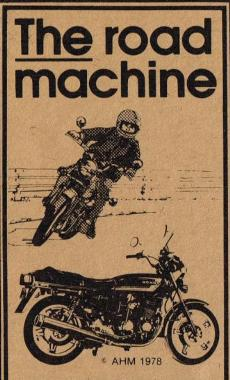
Honda CB-750F Leaning into a curve or cruising along, you'll discover what motorcycling is all about aboard the CB-750F. Features 4-into-1 exhaust system, 736cc 4-stroke transverse OHC 4 with a 5-
