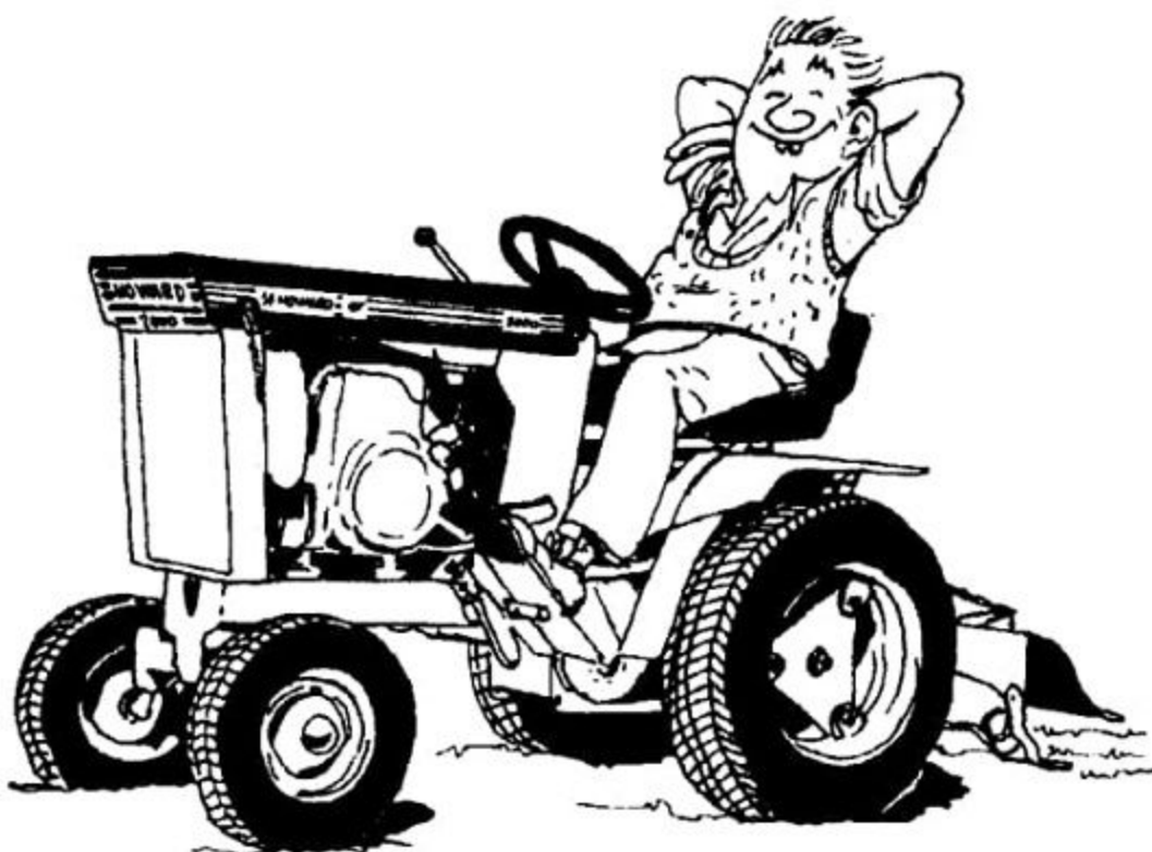
The Howard 2000 compact tractor was first offered in 1962. The 12 HP ride-on garden tractor was a popular machine and had a range of locally built implements to match.
