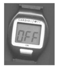
When the monitor is not in use the display screen will show the word "OFF". This indicates the battery is good and the monitor is working
