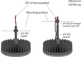
Allows mounting with 1/4"IPS nipple and 1/4-20 all-thread
