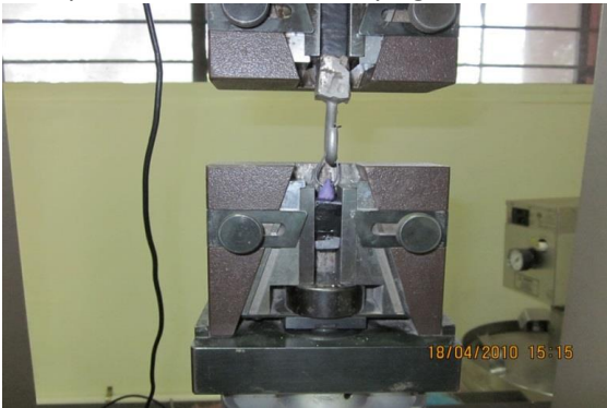
Fig- 2 : Universal testing machine with the specimens fit to the jaws for testing.
