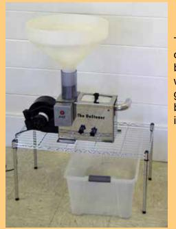
The DeStoner can be mounted on a talbe, wire rack or on a board over the conatiner you want to fill. The wire rack is a good low cost solution. The beans flow through the openings in the wire.
