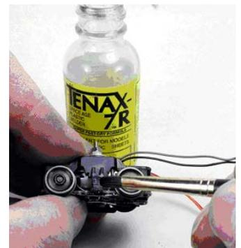
10. Make sure to center the journal boxes both horizontally and vertically to the axle hubs of the Stanton wheels. Look carefully at the photo at right; the mounting sleeves of the side frames are not centered on the side pad of truck. One axle is closer to the center of the drive housing than the other. Mount the frames so that the journals line up with the axles.
