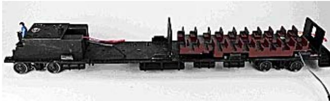
1. Remove the shell by spreading it along the sides. There are four tabs, two on each side.
