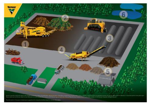
1. Drop-off; 2. Incoming material and grinding; 3. Composting; 4. Screening and finishing; 5. Retail; 6. Drainage pond and perimeter.
