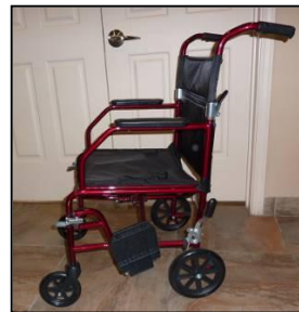
Correct position for front wheels
