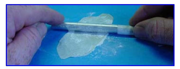
**Step 2 ~ Applying the Milliput.** First you should prepare the surface of the tank by sanding it lightly with course sandpaper. This gives the Milliput something to latch onto. Then lay the putty over the surface and then with a brush (or your finger) dipped in talcum powder you can press the putty down. Then with a sharp hobby knife trim the edges of excess putty.
