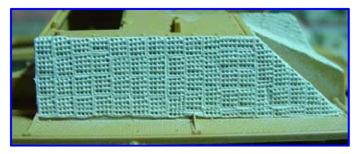
**Step 3 ~ Work on One Section of Milliput at a Time.** Do one area at a time so you don't accidentally touch the still soft putty and damage the pattern.
