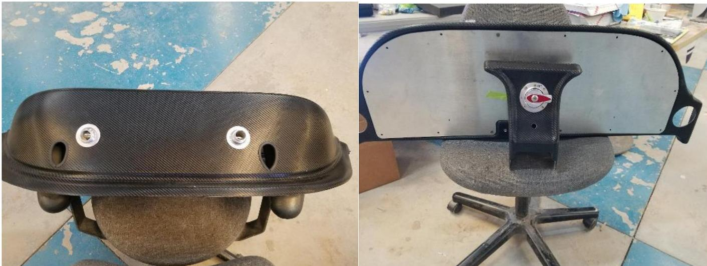
Carbon Fiber Instrument Panel Mount and Fuel Console
