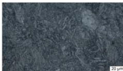
**Figure 7.** Microstructure tempered at 410°C for 3 hours
