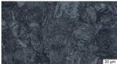
**Figure 10.** Microstructure tempered at 470°C for 2 hours
