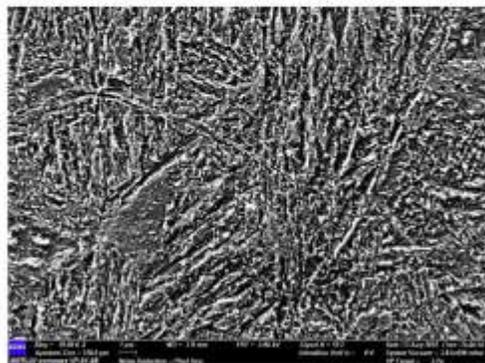
**Figure 12.** Microstructure tempered at 410°C for 2 hours
