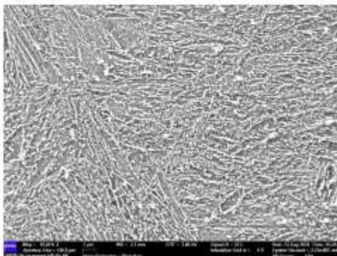
**Figure 13.** Microstructure tempered at 410°C for 3 hours
