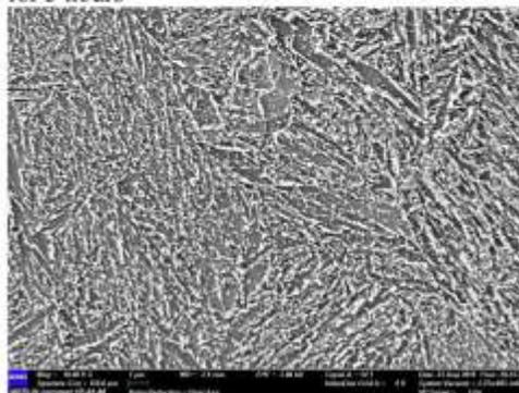
**Figure 17.** Microstructure tempered at 470°C for 3 hours
