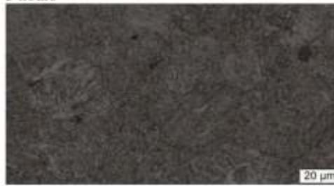
**Figure 11.** Microstructure tempered at 470°C for 3 hours
