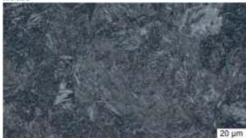
**Figure 8.** Microstructure tempered at 450°C for 2 hours
