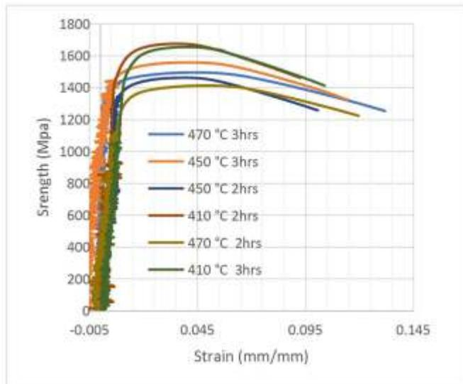
**Figure 19.** Tensile curves of quenched and tempered steel.
