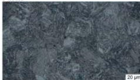
**Figure 9.** Microstructure tempered at 450°C for 3 hours
