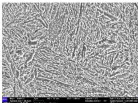
**Figure 14.** Microstructure tempered at 450°C for 2 hours
