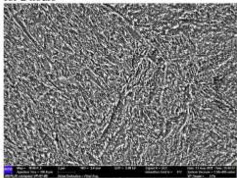
**Figure 16.** Microstructure tempered at 470°C for 2 hours
