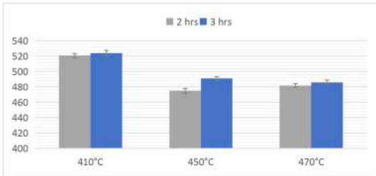
**Figure 18.** Hardness measurements for various tempering temperatures and times
