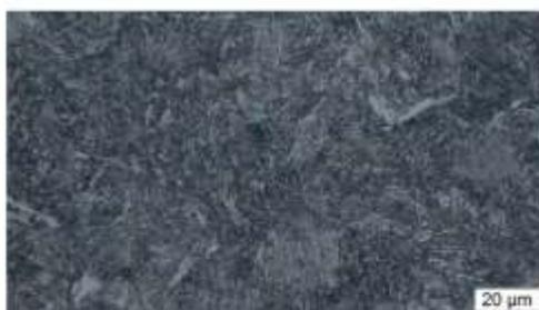
**Figure 6.** Microstructure tempered at 410°C for 2 hours
