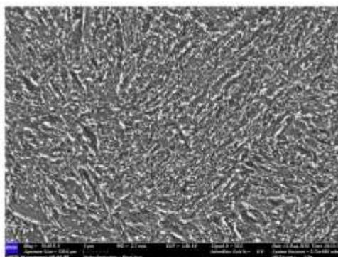
**Figure 15.** Microstructure tempered at 450°C for 3 hours
