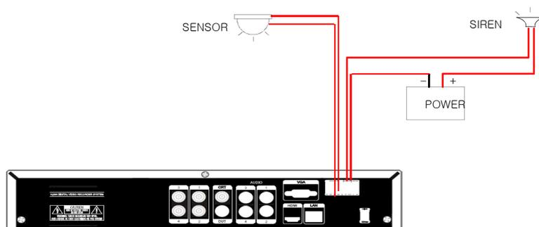
**Sensor In** : Connect the sensors. The sensor are composed of both signal and ground terminals, with a voltage difference of 5V. In the case that the sensor used for input is of the N/O (Normal Open) type, when the voltage difference between the signal and ground falls to 0V (short), the DVR can use this as a trigger to start alarm/sensor based recording.
