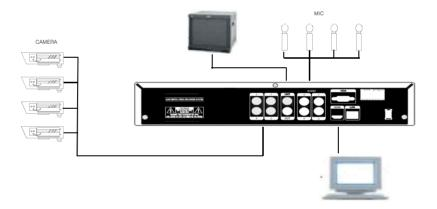
Connect cameras to VIDEO IN by channels. Connect microphone (AMP) to AUDIO IN by channels. Connect VIDEO OUT to VIDEO IN of monitor. Connect HD output to HD Monitor. Connect AUDIO OUT to AUDIO IN of monitor (or speaker). Connect Spot output to Composite Monitor.
