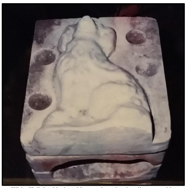
White Hall dog block mold to produce the clay slip cast mold.
