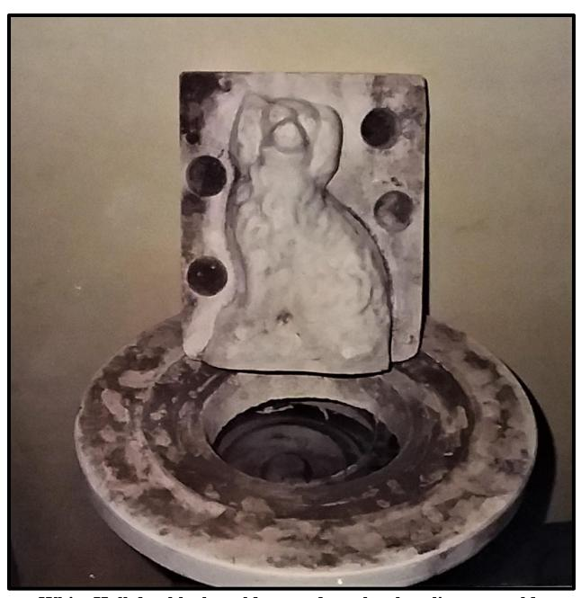
White Hall dog block mold to produce the clay slip cast mold
