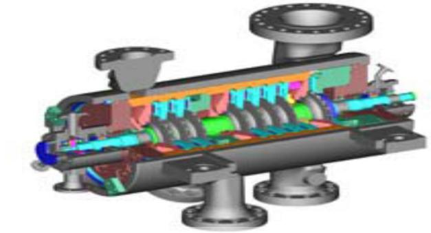
In a Centrifugal Compressor, energy is transferred from a set of rotating impeller blades to the gas.
