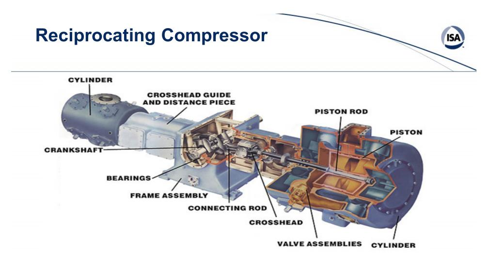
In Reciprocating compressors are positive displacement machines in which the compressing and displacing element is a piston having a reciprocating motion within a cylinder. Reciprocating compressors are often some of the most critical and expensive systems at a production facility, and deserve special attention.
