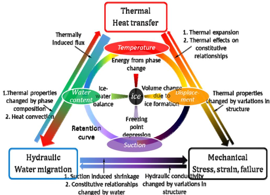
**FIG. 1. Schematic of coupled thermal-hydro-mechanical processes in frozen soil (Liu and Yu 2011).**
