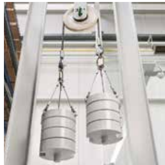
Rope Efficiency Test Facility
