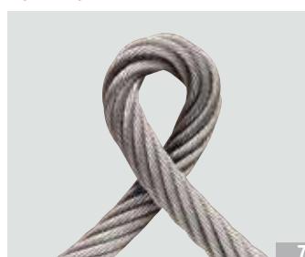
Bend caused by a pinched rope sling
