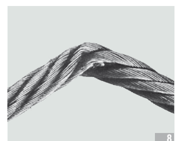
Kind caused by mechanical impact
