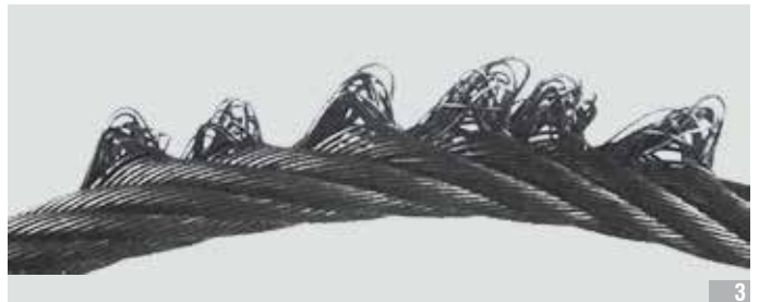
Through corrosion and wear heavy loose strand
