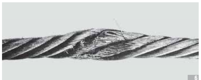
Bend caused by a pinched rope sling
